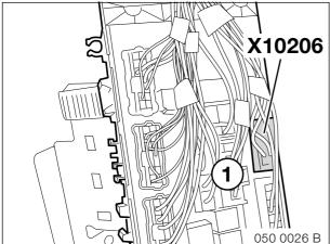
Undo the fuse box (1) and disconnect X10206.
