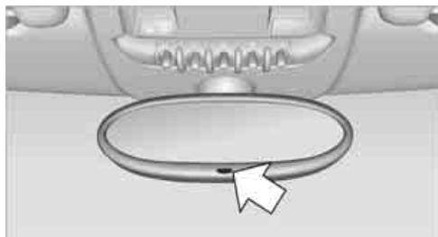
It is controlled by two photosensors:
