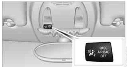
The indicator lamp for the front passenger airbags shows the functional status of the front passenger's front and side airbags in accordance with whether and how the front passenger seat is occupied. The indicator lamp shows whether the front passenger airbags are activated or deactivated.
