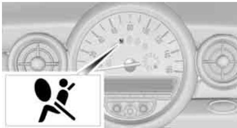
As of radio readiness, page 38, the warning lamp comes on briefly to indicate that the entire airbag system and the belt tensioners are operational.
