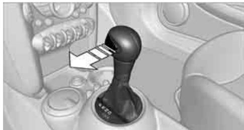
Move the selector lever from position D to the left into the M/S shifting slot: The Sport program is activated and DS is displayed. This position is recommended for a performance-oriented driving style.
