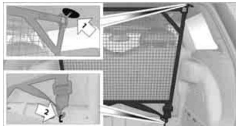
2. Insert each partition net mounting pin all the way into its respective rear mount in the headliner, arrow 1, and push it forward.
