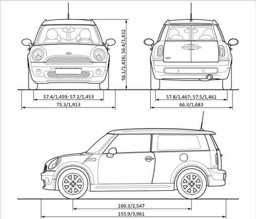
All dimensions in inches/mm. Minimum turning radius  $\varnothing$ : 36 ft in/11.0 m.
