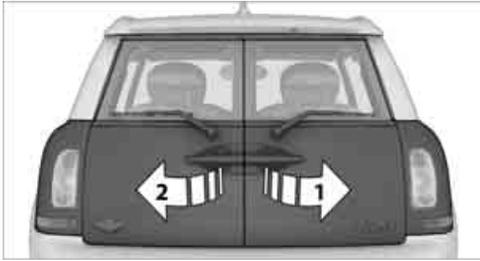
Press and hold the
