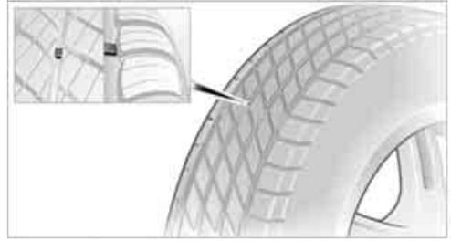
Wear indicators in the base of the tread groove are distributed around the tire's circumference; the letters TWI, for Tread Wear Indicator, on the tire's sidewalls identify tires that incorporate these wear indicators. When tire tread is worn down to the level of the wear indicators, the remaining tread depth is 1/16 in/1.6 mm.
