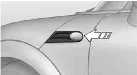
2. Unscrew the bulb holder counterclockwise.
