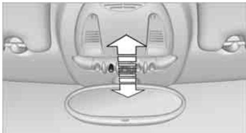
To switch the interior lamps on/off.
