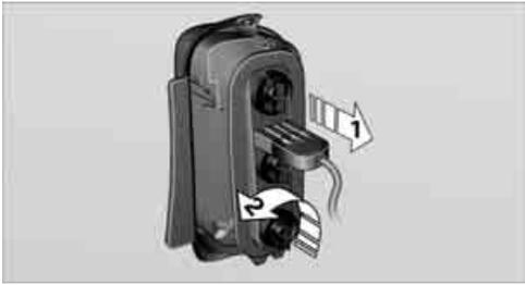
4. Unscrew the corresponding bulb counter-clockwise, arrow 2, and remove it.
