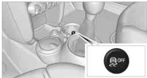
Press the button, the indicator lamp for DTC lights up in the display elements and TRACTION is displayed in the tachometer.
