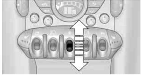
The switch locks or unlocks the doors and Splitdoor when the doors are closed, but the anti-theft system is not activated. The fuel filler flap remains unlocked\*.
