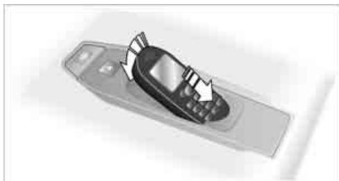
The battery will be charged when the vehicle is at least in radio readiness mode, see the charge display on the mobile phone.
