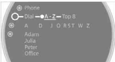
3. To limit the number of entries displayed, select the first letter of the desired entry and press the MINI joystick.
