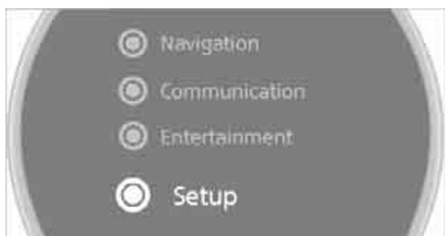
4. Move the MINI joystick to highlight "Setup" and press the MINI joystick.
