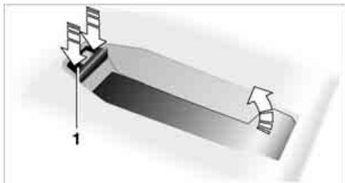
2. Insert the snap-in adapter in the front, arrow 1, and press it downward, arrow 2, until it engages.
