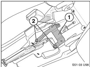
Locate proper position of DSC sensor bracket
