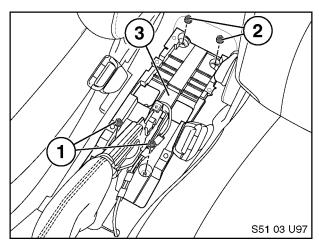
5. Remove front pair (1) and rear pair (2) M6 nuts. Temporarily remove console support bracket (3).
