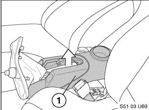
3. Grasp center console (1) and pull upwards to unlock retaining clips.
