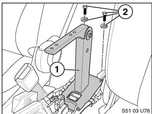
12. Secure armrest base (1) to hex spacers using M6x20mm hex head bolts with M6 split lock washers (2) as shown.
