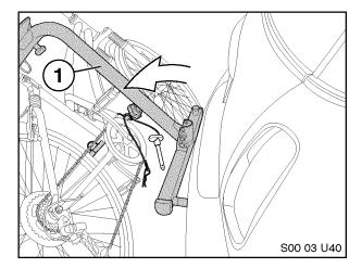
27. Secure lower section of bike frame to rack using nylon straps routed around bike frame and through Tie-Down Strap Arm (6) loops.
