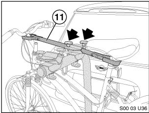
23. Mount bicycle with upper frame tube or frame adapter (11) cradled in Bike Holding Clamp as illustrated.
