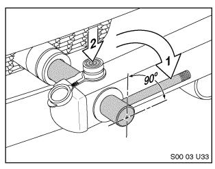
Install Tie-Down Strap Arm (6) onto Pivot Arm (1) as illustrated.
