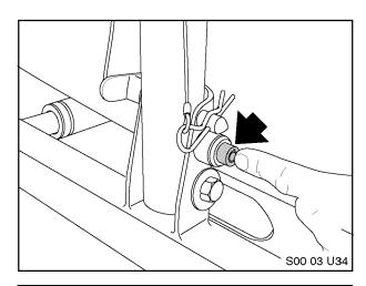
21. To lock Pivot Arm in place push security lock inward as illustrated.
