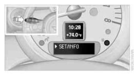
Press and hold the button until the display changes.  Briefly press the button repeatedly until the corresponding symbol and "SERVICE-INFO" are displayed.
