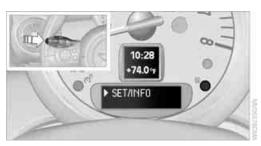
Press and hold the button until the display changes. Briefly press the button repeatedly until the symbol and "SET" are displayed.
