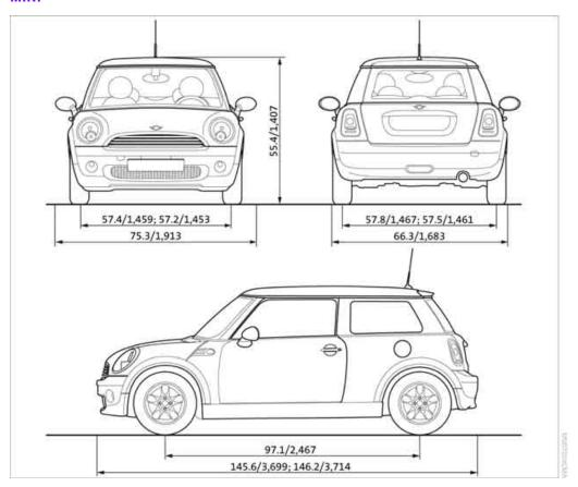
All dimensions given in inches/mm. Smallest turning circle diam.: 35 ft 2 in/10.7 m. Figures following the semicolons: values that differ for the MINI Cooper S.
