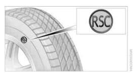
The symbol identifying Run-Flat Tires is a circle with the letters RSC on the sidewall.
