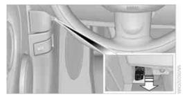
Primary components that make up exhaust emissions can be checked by a device via the OBD socket.
