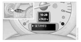
Press and hold the button until the display changes. Briefly press the button repeatedly until the symbol and "SET" are displayed.
