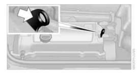
Attach the second terminal clamp of the minus/- jumper cable to the negative terminal of the battery or to the engine or body ground of the vehicle to be started.
