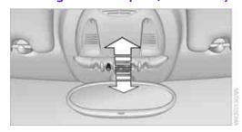
To switch the interior lamps on/off.
