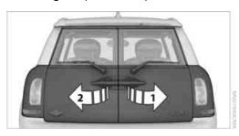
Press the button in the handle or the button of the remote control for an extended time. The splitdoor is unlocked.
