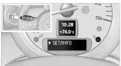
Press and hold the button until the display changes. 4. Briefly press the button repeatedly until the symbol and "SET" are displayed.
