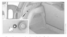
Pull on the green knob with the fuel pump symbol; the fuel filler door opens.
