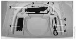
In vehicles with the space-saver spare tire, the tire change set with the onboard tool kit is located beneath the floor mat or level load floor in the cargo bay.
