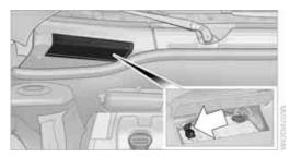
Attach one terminal clamp of the plus/+
