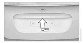
Press the button in the handle, arrow, or the button of the remote control, for an extended period. The tailgate is unlocked and can be opened.
