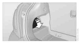
Screw out the desired bulb counterclockwise, arrows 1.
