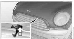
To avoid damage, make sure that the wiper arms are against the windshield before you open the bonnet. ◀
