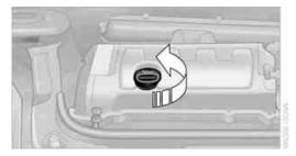
Do not add the maximum quantity of 1 US guart/1 liter of engine oil until the oil level has dropped to just above the lower mark on the dipstick, page 107.
