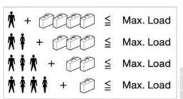
The permissible load is the sum of the occupants' weights and the weight of the cargo. The greater the weight of the occupants, the less cargo/luggage can be transported.
