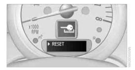
Press and hold the button until the display changes to the first setting. The settings are reset.
