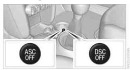
Press the button repeatedly until the indicator lamp for the ASC or DSC comes on. ASC or DSC are deactivated. Stabilizing and drive-output promoting actions are no longer executed.
