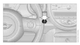
Press the start/stop button to switch radio readiness or the ignition on and off. Do not depress the brake or clutch while doing so.
