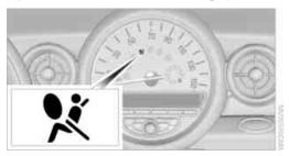
As of radio readiness, page 39, the warning lamp comes on briefly to indicate that the entire airbag system and the belt tensioners are operational.
