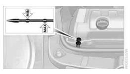
The oil quantity corresponding to the difference between the two marks on the dipstick is 1 US quart/1 liter.
