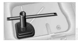
Screw the lifting handle from the onboard tool kit onto the thread.
