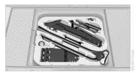
Your vehicle comes with an onboard tool kit that varies with the equipment version; it is stored underneath the level load floor.
