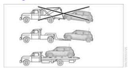
Have the MINI transported with a tow truck with a so-called lift bar or on a flat bed.
