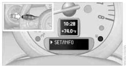
Press and hold the button until the display changes. 4. Briefly press the button repeatedly until the symbol and "SET" are displayed.
