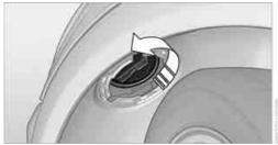
4. Screw out the bulb counterclockwise.
