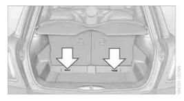
There are two additional anchors for childrestraint systems with tether straps, arrows. When the vehicle is equipped with a level load floor\*, the anchors are covered. Their positions are labeled.
