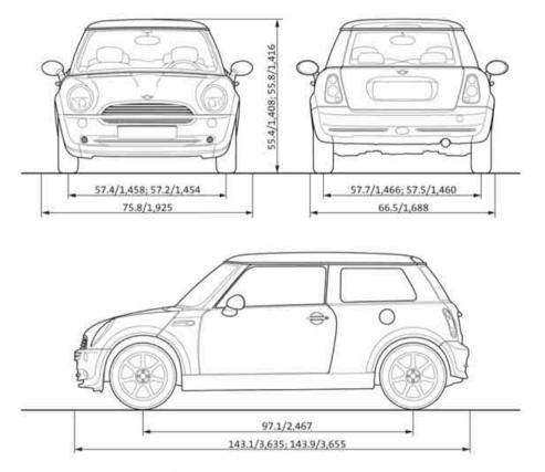
All measurements in inches/millimeters. Smallest turning circle dia. 34 ft 10 in/10.66 m. Values following a ; are differing values for MINI COOPER S. 0462BCMA
