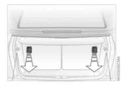
Pull the lever to release the catch
