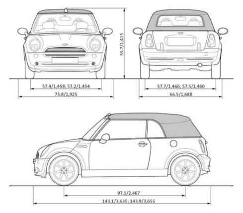
All measurements in inches/millimeters. Smallest turning circle dia. 34 ft 10 in/10.66 m. Values following a ; are differing values for MINI COOPER S.
