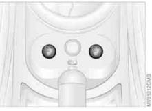
Press once for each temperature level. The highest preselected temperature is set when two LEDs are lit.
