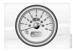
Do not operate the engine with the needle in the red overspeed zone of the gauge.
