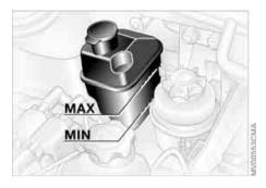
As an example, the illustration shows the coolant tank of the MINI COOPER and the MINI COOPER Convertible.
