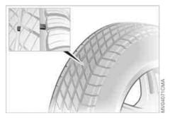
Wear indicators in the tread-groove base are spread around the circumference of the tire and are marked on the sidewall of the tire with TWI, Tread Wear Indicator. When tire tread is worn down to the level of the wear indicators, the remaining tread depth is 1/16 in/1.6 mm.
