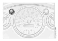
To control the instrument lighting, press the button.
