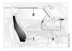
The following airbags are located under the marked covers:
