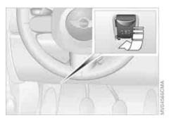
Primary components of exhaust emissions can be checked by a device via the OBD socket.
