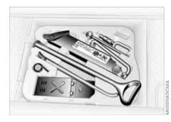
The picture shows as an example the tire change set with onboard tools for vehicles with the space-saver spare tire.
