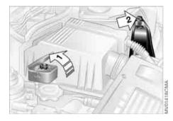
The illustration shows the auxiliary jumpstarting terminal on the MINI COOPER S and the MINI COOPER S Convertible. In the MINI COOPER S and the MINI COOPER S Convertible, the auxiliary jumpstarting terminal, arrow 1, acts as the positive battery terminal, refer to view of engine compartment on page 120. The cover is marked with a +.
