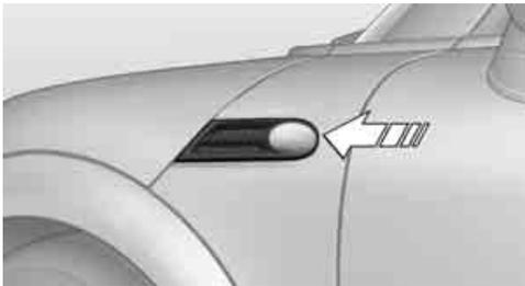
2. Unscrew the bulb holder counterclockwise.
