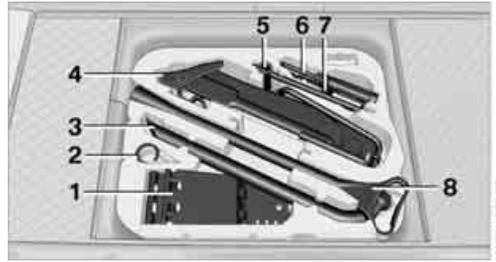
On vehicles with a space-saver spare tire, the tire change set with onboard tools is stored under the floor mat in the cargo area.
