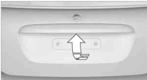
Press the button in the handle, arrow, or the
