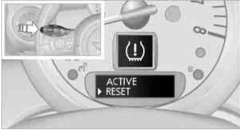
5. Press and hold the button until "RESETTING" is displayed.
