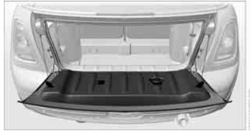
▷ The maximum load that may be placed on the open tailgate is 175 lbs/80 kg. ◀
