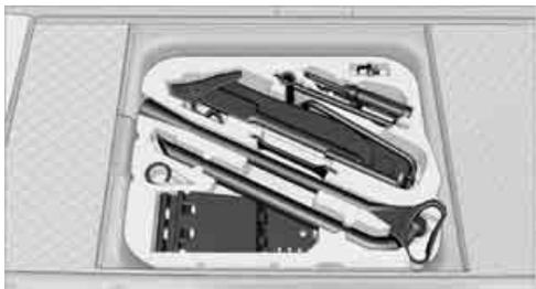
Your vehicle comes with an onboard vehicle tool kit that varies with the equipment version; it is stored underneath the flat load floor.
