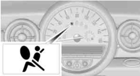
As of radio readiness, page 44, the warning lamp comes on briefly to indicate that the entire airbag system and the belt tensioners are operational.
