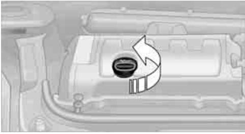
Do not add the maximum quantity of 1 US quart/1 liter of engine oil until the oil level has dropped to just above the lower mark on the dipstick, page 128.
