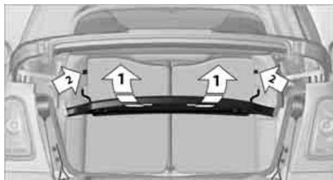
1. Pull the lever, arrow 1, and fold the rear seat backrest forward.
