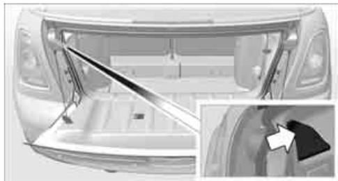
2. Pull on the green knob with the fuel pump symbol. The fuel filler flap is released.
