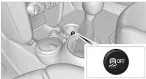
Press the button for at least 3 seconds: the DSC indicator lamps in the display elements come on. The Dynamic Traction Control DTC and Dynamic Stability Control DSC are both deactivated. There will be no more stabilizing interventions.
