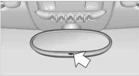
It is controlled by two photosensors:
