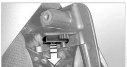
Using the Allen wrench, loosen second bolt, arrow, to unlock the convertible top.
