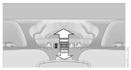
To switch the interior lamps on/off.
