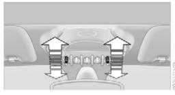
To switch the reading lamps on and off. Press the switch.
