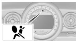
As of radio readiness, page 60, the warning lamp lights up briefly to indicate that the entire airbag system and the belt tensioners are operational.
