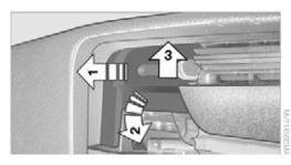
Pull out the sensor from cover, arrow, and place on the inner side panel.
