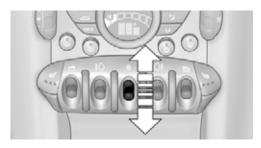
The switch locks or unlocks the doors and tailgate when the doors are closed, but the antitheft system is not activated. The fuel filler flap remains unlocked.
