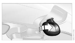
Using the handle, push unlocked convertible top upwards and open about six inches.
