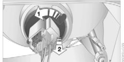
Push on the catch, arrow 1, and disconnect the connector, arrow 2.
