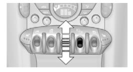
Turn on front fog lamps:Press the switch upward
