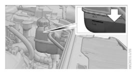
The coolant level is correct if it is between the marks.
