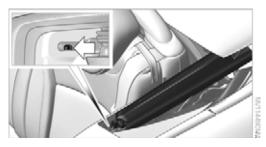
Slide cover in travel direction, arrow 1, and rotate out sideways, arrow 2. If necessary, press plastic trim, arrow 3 slightly inward.
