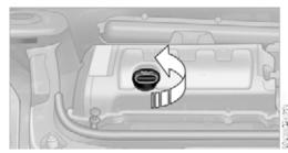
Do not add the maximum quantity of 1 US guart/1 liter of engine oil until the oil level has dropped to just above the lower mark on the dipstick, page 222.
