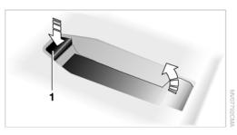
Insert the snap-in adapter at the front, arrow 1, and press downward, arrow 2, until it clicks into place.
