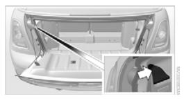
Move the convertible top to its uppermost position, refer to Loading aid page 117, and remove the cover of the luggage compartment side wall.
