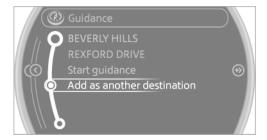
Select the location where the intermediate destination is to be inserted.
