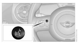
A This symbol on the Control Display and an acoustic signal indicate that the voice activation system is ready to receive spoken commands.
