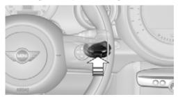
Insert the key all the way into the ignition lock. Radio readiness
