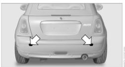
The mounting points are under the protective caps in the bumper.
