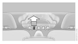
Push switch back to open the convertible top. The windows open during this procedure.
