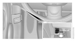
The primary components that make up the emissions can be checked by a device via the OBD socket.
