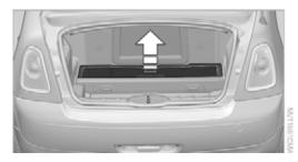
Using the Allen wrench from the tool kit, turn the gold-colored screw, see arrow, in the direction of the arrow by about four or five rotations all the way to the stop.
