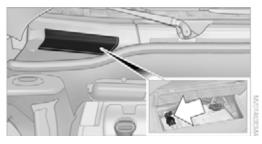
Release the tabs on the left and right sides of the positive terminal cover, arrows 1, and lift the cover to open, arrow 2.
