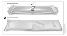
Fold the wind deflector 1 closed and slide it into the storage pouch 2.
