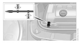
The oil quantity corresponding to the difference between the two marks on the dipstick is 1 US quart/1 liter.
