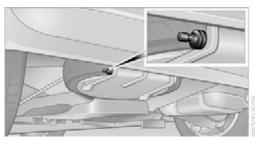
A valve extension for checking the inflation pressure is located behind the bumper.
