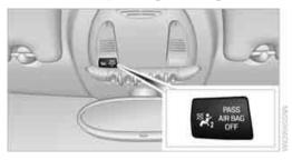
The indicator lamp for the front passenger airbags shows the functional status of the front passenger's front, side, and knee airbags in accordance with whether and how the front passenger seat is occupied. The indicator lamp shows whether the front passenger airbags are activated or deactivated.
