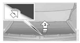
Lift up load floor behind and fold forwards,
