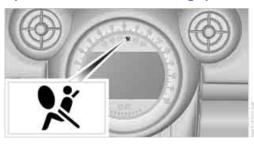
As of radio readiness, page 48, the warning lamp lights up briefly to indicate that the entire airbag system and the belt tensioners are operational.
