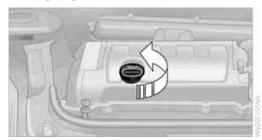
Do not add the maximum quantity of 1 US quart/1 liter of engine oil until the oil level has dropped to just above the lower mark on the dipstick, page 203.
