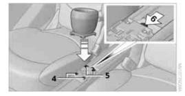
First insert the cupholder into the front mounts 4 and then snap it into the rear mounts 5.
