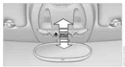
To switch the interior lamps on/off.
