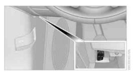
The primary components that make up the emissions can be checked by a device via the OBD socket.
