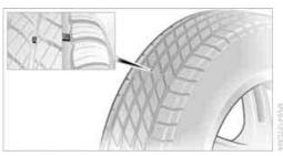
Wear indicators in the base of the tread groove are distributed around the tire's circumference: the letters TWI, for Tread Wear Indicator, on the tire's sidewalls identify tires that incorporate these wear indicators. If the tire tread has been driven down to the wear indicators, a tread depth of 0.063 in/1.6 mm has been reached.
