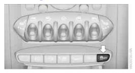
Press the button for at least 3 seconds; the indicator lamp DSC OFF on the speedometer comes on and DSC OFF is displayed on the tachometer. The Dynamic Traction Control DTC and Dynamic Stability Control DSC are both deactivated. There will be no more stabilizing interventions.
