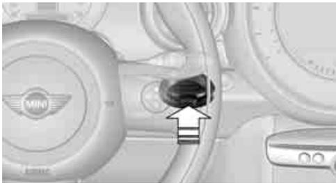
Insert the key all the way into the ignition lock.
