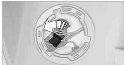
5. To insert the new bulb and replace the cover, proceed in reverse order.
