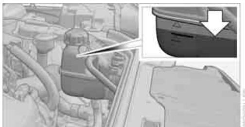
The coolant level is correct if it is between the marks.
