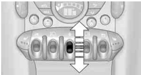
The switch locks or unlocks the doors and tail-gate/Split Rear Barn Doors when the doors are closed, but the anti-theft system is not activated. The fuel filler flap remains unlocked.
