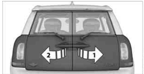
Press and hold the button in the handle or the **⏏** button for the remote control for approx. 1 second. The Split Rear Barn Doors are unlocked.
