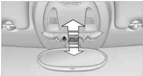
To switch the interior lamps on/off.
