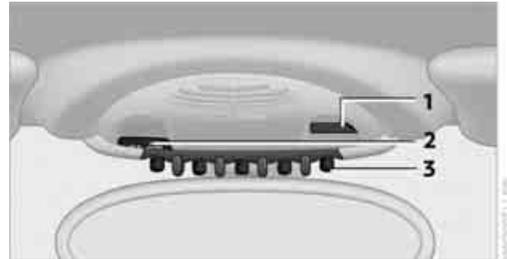
**1** Microphone for voice activation system and for telephone in hands-free mode**2** Indicator/warning lamp for front passenger airbags 79**3** Switch panel
