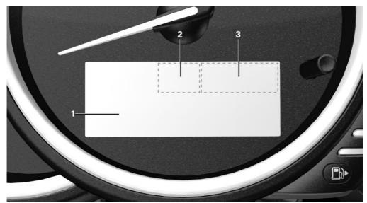
Driver assistance systems Messages, for instance Check Control Time 95 External temperature 95 Selection lists 99 Total miles/trip odometer 95
