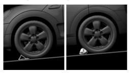
If you need to change a wheel on a slight downhill gradient, place chocks and other suitable objects, for example a rock, under the wheels of both the front and rear axles against the rolling direction.
