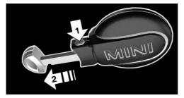
Press the button, arrow 1, and pull out the integrated key, arrow 2.
