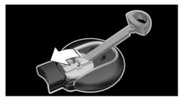
4. Push battery in the direction of the arrow using a pointed object and lift it out.
