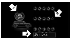
The display of the MINIMALISM analyzer consists of a fish in a water glass riding along on the roof of a MINI and a table of values. The fish and the movements of the water in the glass, arrow 1, symbolize the efficiency of the driving style.
