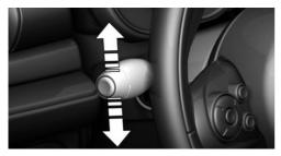
With the ignition switched off, press the lever either up or down past the resistance point.
