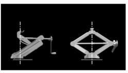
Make sure that the vehicle jack foot stands vertically and perpendicularly beneath the jacking point after extending the vehicle jack.
