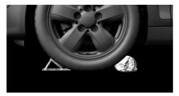
Place wheel chocks or other suitable objects in front and behind the wheel that is diagonal to the wheel to be changed.
