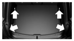
With storage package: to secure the cargo there are four lashing eyes in the cargo area.
