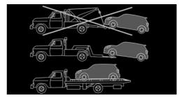
Your vehicle should be transported with a tow truck with a so-called lift bar or on a flat bed.
