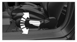
Pull the lever up or press it down as often as needed to reach the desired height.
