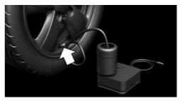
5. With the compressor switched off, insert the plug into the power socket inside the vehicle.
