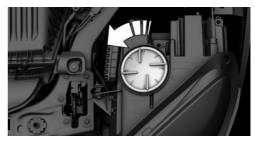
Turn the bulb holder counterclockwise, arrow 1, and remove, arrow 2.
