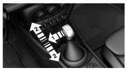
Press the selector lever to the left out of selector lever position D, arrow 1. Next, push the selector lever forward or pull it backward, arrow 2.
