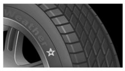
For each tire size, the manufacturer of the vehicle recommends certain tire brands. These can be identified by a star on the tire sidewall.
