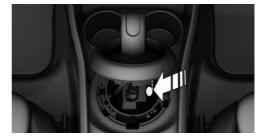
Move the selector lever slightly toward the rear; to do this press the button on the front of the selector lever.
