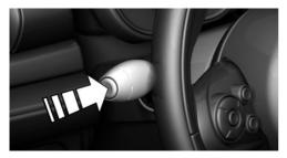
Press and hold button on signal lever.
