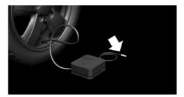
5. With the ignition turned on or the engine running, switch on the compressor.
