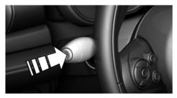
Press and hold button on blinker lever.
