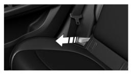
Pull the strap and apply your weight to the backrest or lift it off, as necessary.
