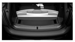
2. Grasp the MINI Picnic Bench in the middle and pull it back and up against the force of the magnets.
