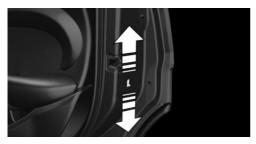
Push the locking lever on the rear doors up. The door can now be opened from the outside only.
