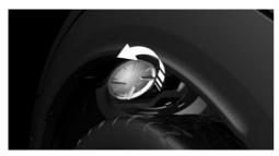
4. Tilt the bulb holder down, arrow 1, and pull it downward out of the headlight, arrow 2.
