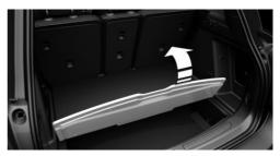
2. Place the MINI Picnic Bench on the part of the cargo area floor that is folded over and attach it using the four snaps.
