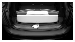
Fold the rear part of the cargo area floor downward and place the MINI Picnic Bench over the loading lip of the cargo area. Place a protective cloth over the bumper.
