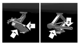
Insert the vehicle jack into the rectangular recess of the jacking point closest to the wheel to be changed.
