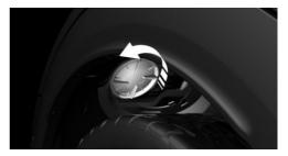
4. Turn the bulb holder counterclockwise, arrow 1, and remove, arrow 2.
