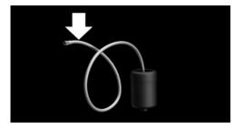
Slide the sealant container into the holder on the compressor housing, ensuring that it engages audibly.
