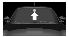
The camera is installed near the interior rearview mirror.
