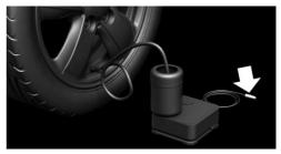
6. With the ignition turned on or the engine running, switch on the compressor.
