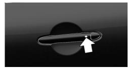
Press and hold down the handle of the driver or the front seat passenger.
