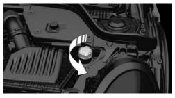
The coolant level is correct if it lies between the minimum and maximum marks in the filler neck.
