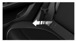
Pull the strap forward. The rear seat backrest folds forward.
