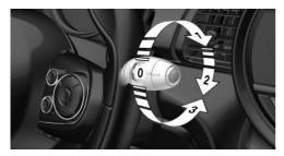
Turn the switch from idle position 0 upward, arrow 1: interval mode. When reverse gear is engaged, the system switches to continuous operation.
