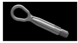
The screw-in tow fitting should always be carried in the vehicle.
