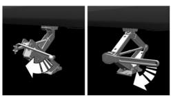
Take your hand away from the jack as soon as the vehicle jack is under load and continue turning the crank or lever with one hand. 5. Make sure that the vehicle jack foot is extended vertically.
