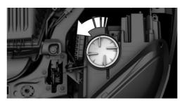
Tilt the bulb holder up, arrow 1, and pull it out of the headlight toward the rear, arrow 2.
