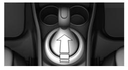
Lift the sleeve. Unplug the cable connector, if needed. Using the screwdriver from the onboard vehicle tool kit, refer to page 257, press the yellow release lever downward, see arrow.
