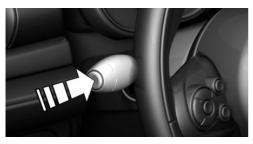
Press and hold button on signal lever.
