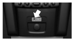
The USB interface and the AUX-IN port are located at the front in the center console.
