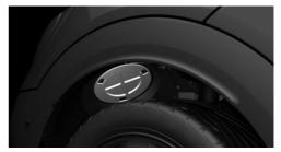
Unscrew the inner cover counterclockwise, and remove it.
