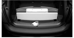
Fold the rear part of the cargo area floor downward and place the MINI Picnic Bench over the loading lip of the cargo area. Place a protective cloth over the bumper.
