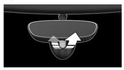
To reduce the blinding effect of the interior mirror, flip the lever forward.
