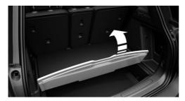
Place the MINI Picnic Bench on the front part of the cargo floor panel and attach it to the rear part of the cargo floor panel using the four snaps.
