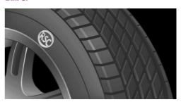
The tires are marked on the tire sidewall with RSC Run-flat System Component.
