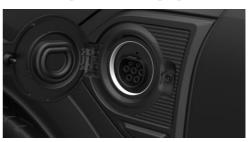
An indicator light is located on the charging socket.
