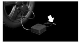
With the ignition switched on or the engine running, switch on the compressor. If a tire inflation pressure of at least 2 bar cannot be reached, contact your dealer's service center or another qualified service center or repair shop.
