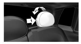
To fold down: press the button, arrow 1, and press down the head restraint, arrow 2. ▶ Forward: fold the head restraint toward the front as far as it will go. Make sure that the head restraint engages correctly.
