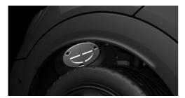
Unscrew the inner cover counterclockwise, and remove it.
