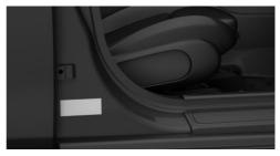
The vehicle identification number can be found on the type label, on the right-hand side of the vehicle.
