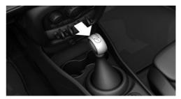
Move the selector lever into the desired position.
