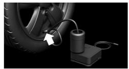
With the compressor switched off, insert the plug into the power socket inside the vehicle.
