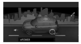
Example: residential area or area with low speed restrictions. ePOWER electric driving is being prepared. When the residential area is reached, electric driving takes precedence.
