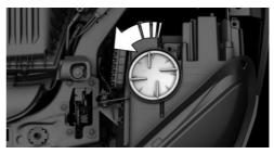
Turn the bulb holder counterclockwise, arrow 1, and remove, arrow 2.
