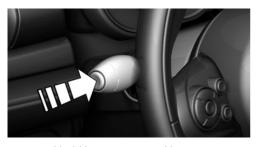
Press and hold button on signal lever.
