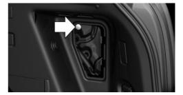
Briefly press the rear edge of the fuel filler flap. Fuel filler flap is opened.
