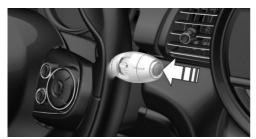
Press the button on the wiper lever.
