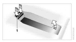
2. Insert the snap-in adapter in the front, arrow 1, and press it downward, arrow 2, until it engages.
