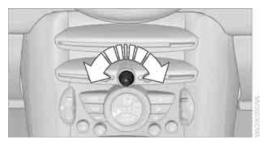
Rotate the button while a message is being voiced.
