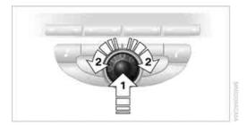
1. Turn the rotary button, arrow **2**, to select a function by marking it, e.g. "PHONE".
