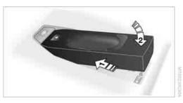
3. To remove the snap-in adapter, press area 1 surrounding the button.
