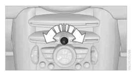
To adjust the volume of the hands-free sound system and the ringing tone, rotate the button while sound is being issued.
